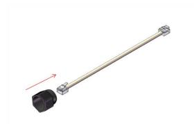
4. Slide the GM67X-CS-R or GM67X-CS-B seal into GM67X-CS-R or GM67X-CS-B body as shown.
